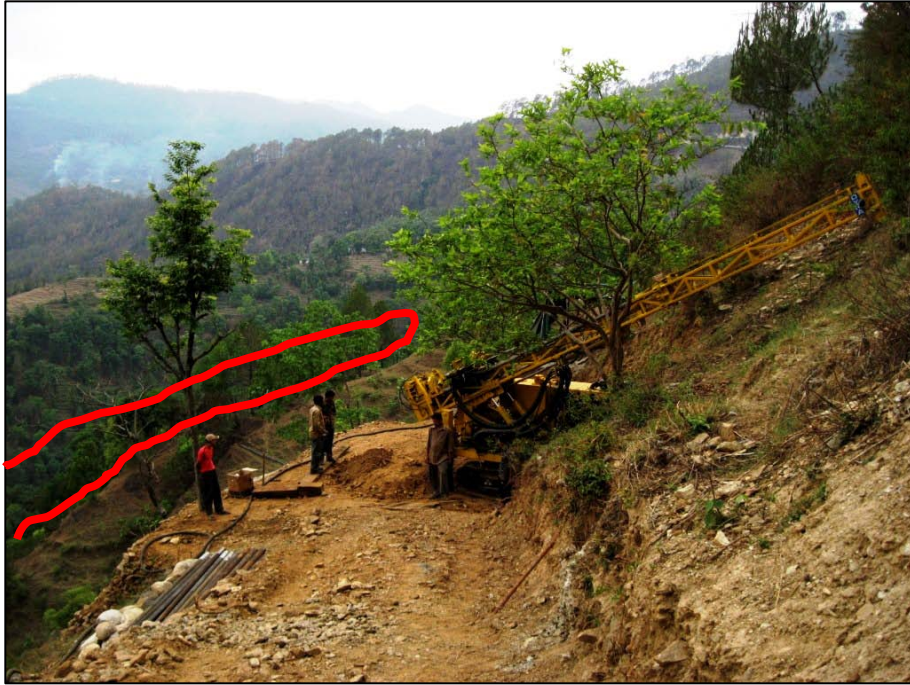
Askot Project, Uttarakhand, India. DDH 10AA018 drill site, view west, showing location of EM and soil geochemical anomaly in red – an extension along strike northwest of the known Askot mineralization. Dip of extension is 70^\circ toward the drill. Drill is in process of setting up. May 5, 2010.
